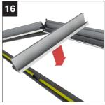
If the project contains side rafters: Locate the rafter on the bolts at the ridge and eaves, once in position secure with flanged nuts. Check the ridge is level.
