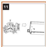
Fit each hip rafter to the tenons of the ridgeLOCK. Secure in place into pre drilled holes using M5 x 16mm screw in the upper hole and the M5 x 20mm screw in the lower hole.
