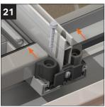
Ensure that glazing end profile sits snugly behind grommet, on the glazing end stop. Now using the fixings provided, screw down into the rafters as shown.
