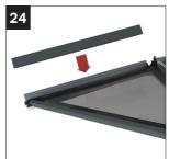
Work your way around the roof and fit the rafter top caps.
