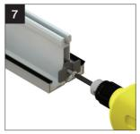
Attach the glazing rafter end cap brackets - as access restriction may prevent easy fixing later.
