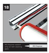
Seal underside of top face of glazing end profile as shown. Depending on the roof specification this can either be a PVCu or Aluminium profile.
