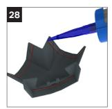
Apply a small bead of sealant to the inside of the external cover (as shown) around where the part meets the glazing rafters top caps and the ridge top cap.
