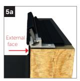
Cross section of timber kerb with eaves beam/rail in position - note flush with outer edge of kerb.
